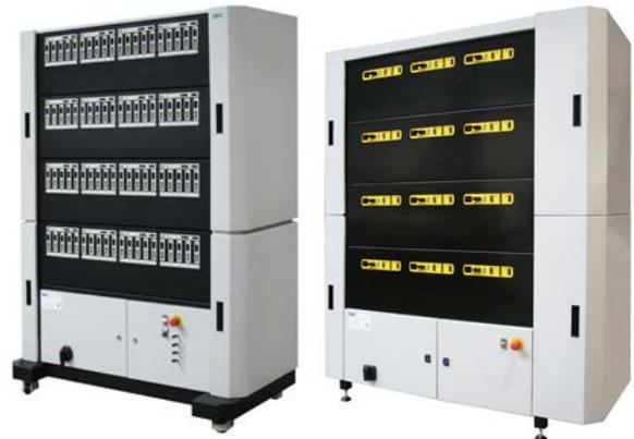
ACT0550 cell tester (left) and SBT10050 module tester (right)
